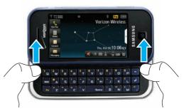
When you slide the phone open, the display rotates from a vertical viewing mode to a horizontal viewing mode.
