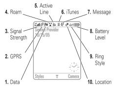
1 Data Indicator – Shows connection status. The Bluetooth® wireless connection indicator ≱ shows when a Bluetooth connection is active. Other indicators can include:
