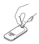
To release and replace the back cover, turn the screw with a coin or screwdriver.
