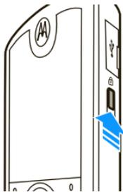
**key all the way down to the bottom power ON/OFF position.**
